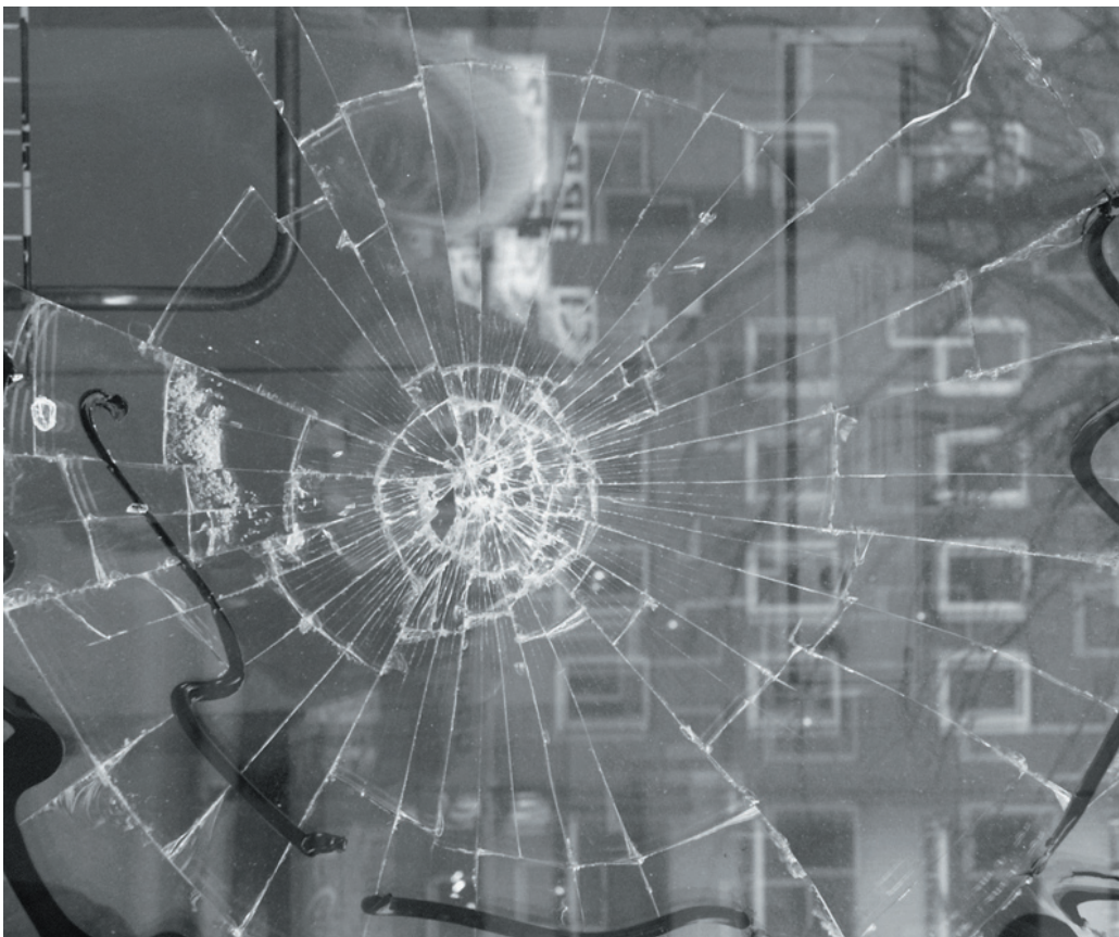
Figure 2. Impact stress crack pattern The photo shows a cracked glass window pane where circumferential cracks have formed due to impact stress.
